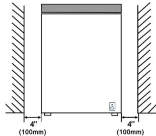
Make sure that sufficient room is provided around the appliance to ensure free air circulation.
